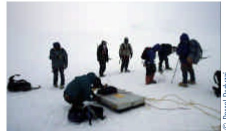
Christian Herold prepares the ground penetration radar before undertaking measures at more than 6000 meters above sea level. The large white device with batteries and laptop weight together 35kg. Cold and windy conditions requested special protection measures for the electronic equipments.
